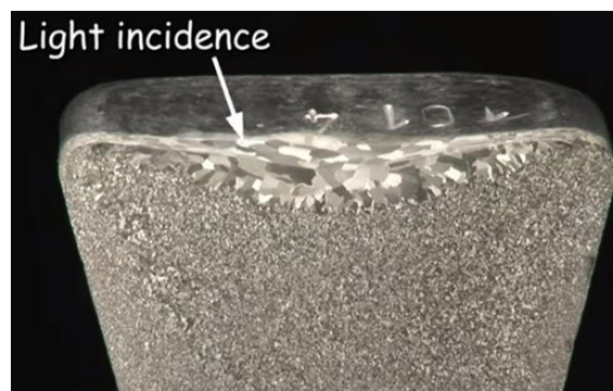
Fig. 2.1.41 Grain Boundary Assessment after Chemical Polishing for Stainless Steel
