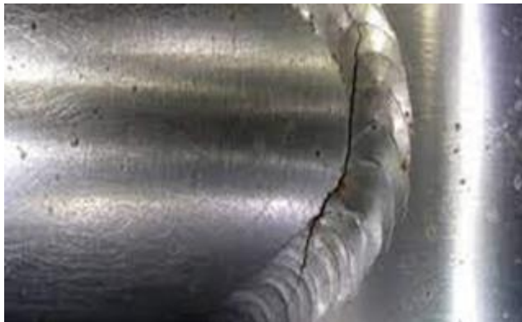
3.2.28. ábra: Repedés. Forrás: https://www.rapiddirect.com/blog/types-of-welding-defects/
